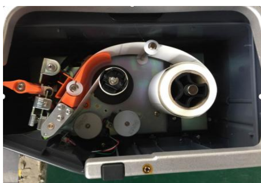
f. Press [↑] button to roll the label paper
